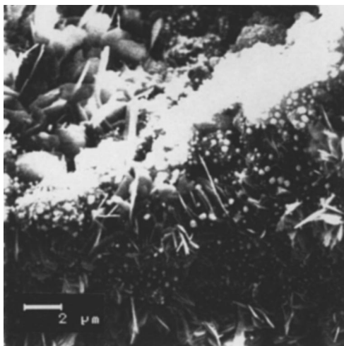
Fig. 5. SEM picture of the layer of washcoat onto the metallic substrate (Fig. 4) after hydrothermal treatment at 900°C for 270 h in steam.
